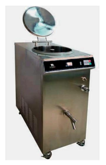
Thermal insulated lid made by sandwich two stainless steel sheet with insulate material at the middle, could save energy and offer safer operation.
