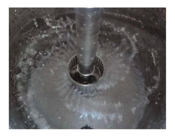
Demonstrate the performance by water. Rotor sucks down mix and cut ingredient into smaller size and squeeze the liquid mix through small holes for emulsification and then mix return to the mix surface , and then sucked down again for next cycle
