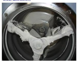
Almost no gelato left on beater or cylinder after extrusion, no loss when changing flavor.
